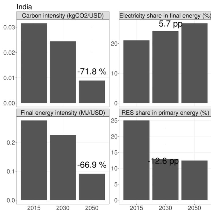
Figure 3: Decarbonisation indicators for the 2 °C scenario (starting from NDC emission levels in 2030). Numbers in graph indicate change between 2015 and 2050 (intensity indicators: %, share indicators: percentage points, pp)
